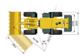
► Note: the above dimensions are based on the standard configuration.
